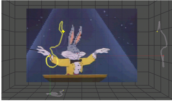
Figure 1. An author edits a haptic motion path to match the movement of the animated character's hand. The path is projected onto the right and bottom walls for precise positioning.
